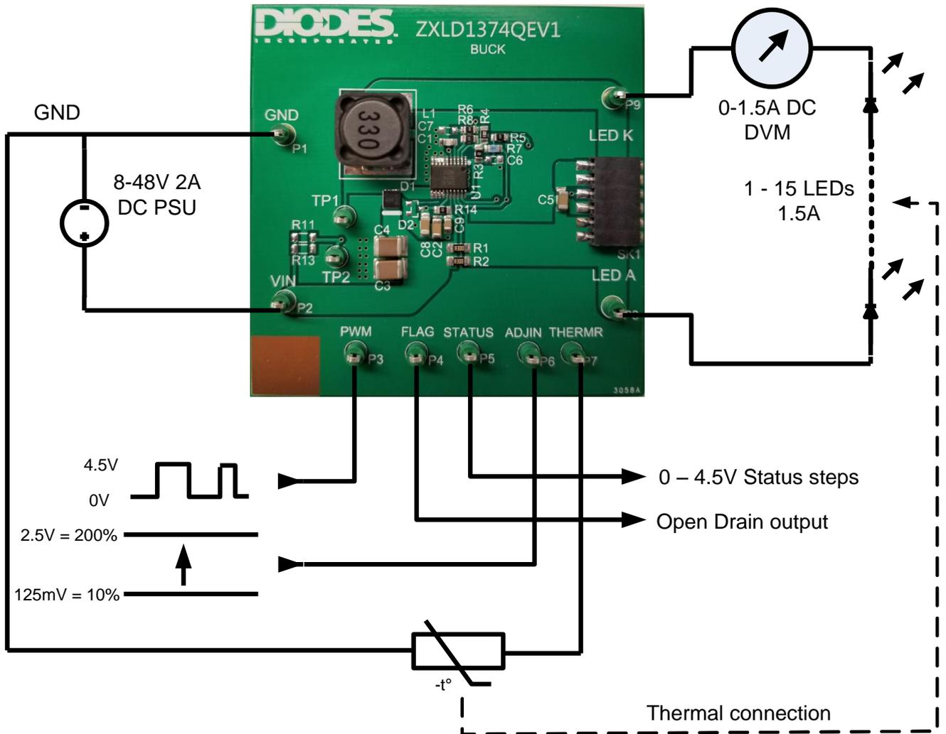
Fig. 1 ZXLD1374QEV1 Evaluation board connection diagram
